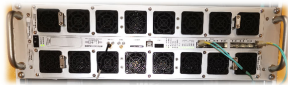
Figure 4: DBPM3 front side with two rows of eight fans.
