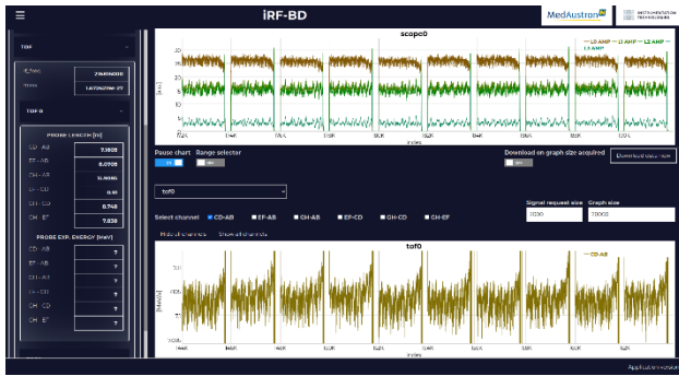
Figure 5: Amplitude and TOF measurement with “local” web user interface.
