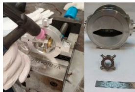
Figure 13: The welding process(left), the current BPM size and the new BPM (right).
