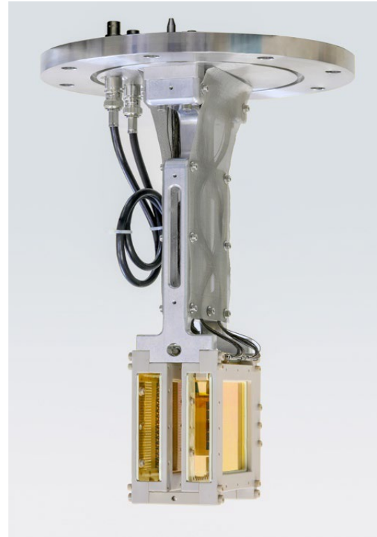
Figure 2: PEPITES sensitive area (gold) mounted on its support tool (see text).
