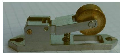
Figure 1: Roller contact for grounding probe structure.
