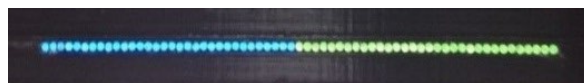
Figure 2: The two fibre types glued into 3D prints. The scintillating fibre area consists of (a) 32 blue fibres (channel 0 – 31) and (b) 32 green fibres (channel 32 – 63).
