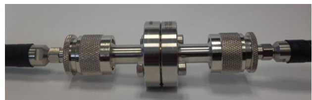
Figure 4: Photo of setup to measure reflection of two feedthroughs.
