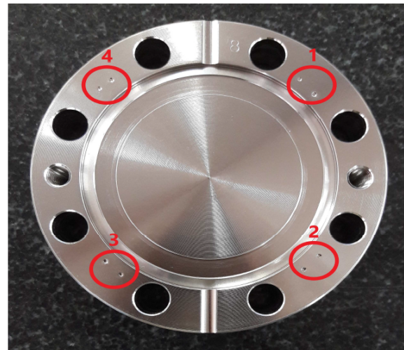
Figure 7: Hardness measurements of 316 LN ESR before and after heat treatment with 1110 °C at four different position on the flange. The values are in Brinell Hardness (HB).
