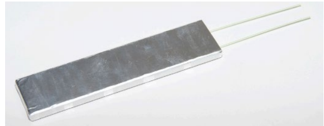
Figure 3: Plate scintillator assembly based on the EJ-204 scintillator and the BCF-92 wavelength shifting fiber, wrapped in foil.
