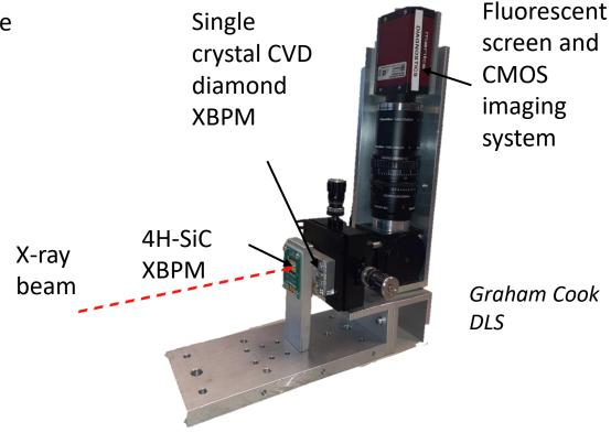
The two XBPMs were mounted in series with the camera upstream, the whole detector system was mounted on a x-y motion stage.
