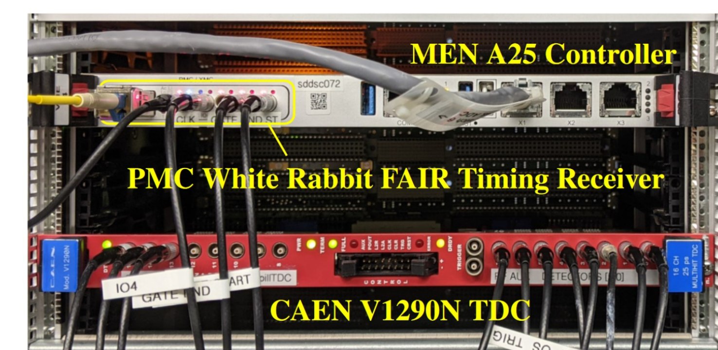
Fig. 2: VMEbus mainframe configuration
