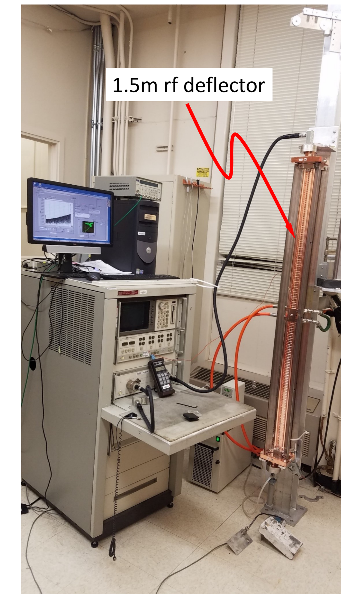
Final beadpull measurements of new 1.5 m rf deflector
