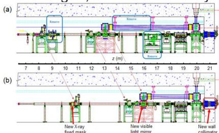
Figure 1: Profile of components in 35-BM front end [3]. The longitudinal coordinate  $z$  is with respect to the bending nominal bending magnet photon source point. (a) Existing APS configuration. (b) Proposed APS-U configuration. For APS-U, a section of the visible light telescope, the pinhole aperture assembly and pinhole camera will be removed.
