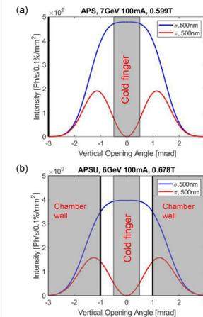
Figure 3: Calculated angular distribution of visible synchrotron radiation and angular apertures in the beamline in the vertical plane [4]. Beam parameters are summarised in Table 2. (a) Calculated flux at 500 nm for APS. (b) Calculated flux at 500 nm for APS-U. Implementation of a cold finger for the APS-U storage ring would significantly reduce the visible photon flux.
