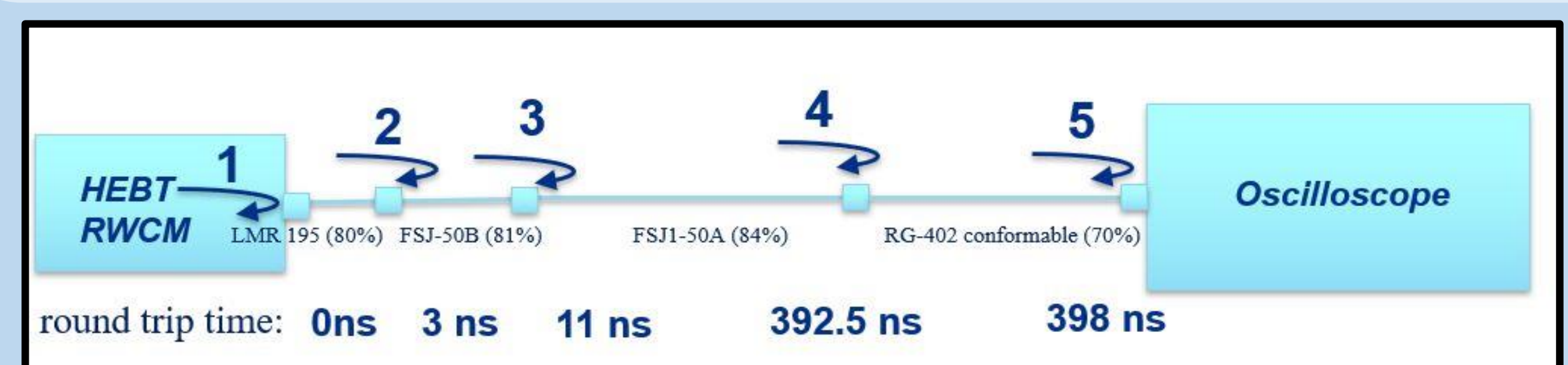
Figure 4: Cabling between the RWCM and the oscilloscope
