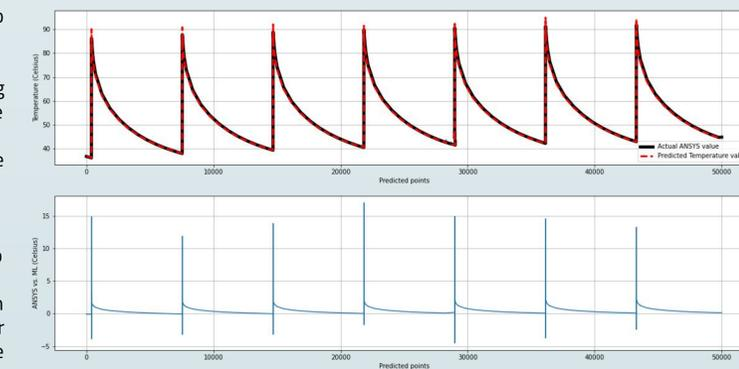
FIG.4 - (Top) Comparison between temperature values calculated in ANSYS and those predicted by the ML-based method. (Bottom) Temperature difference between the ANSYS and the ML-results.
