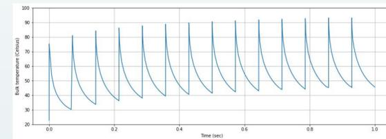
FIG.1 - Temperature as a function of the time, calculated in ANSYS for the graphite bulk of the SPK IBS (50µs long proton pulses, 6 mA, 14 Hz and 73 MeV).
