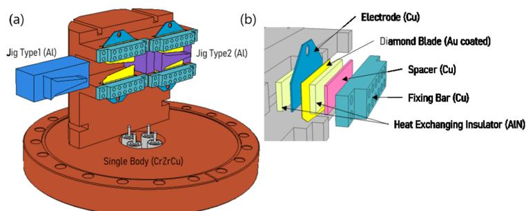
Figure 1: (a) A schematic diagram of the structure of the pick-up of EPU-PBPM. (b) Layered construction of blades.
