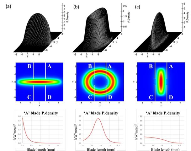
Figure 2: The power density according to the light polarization. (Top) 3D wire-frame. (Middle) 2D contour plot. (Bottom) Power density for 'A' blade. (a) is for horizontal linear mode, (b) is for circular mode, and (c) is for vertical linear mode.
