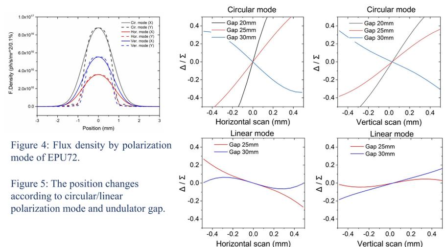
Figure 4: Flux density by polarization mode of EPU72.
