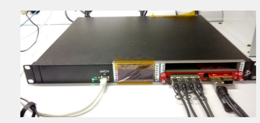
Prototype of FOFB platform: \mu\text{TCA} crate + FPGA board (with SOC) + FMC cards for SFP and serial interfaces
