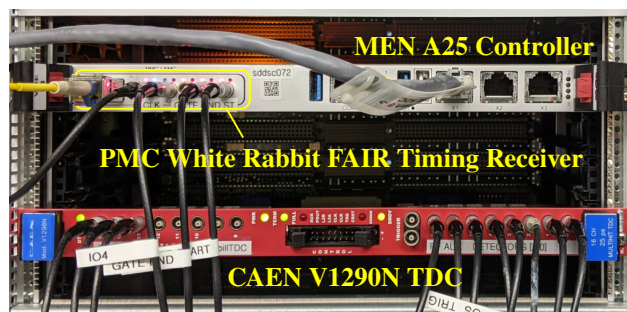
Figure 2: VMEbus mainframe configuration.
