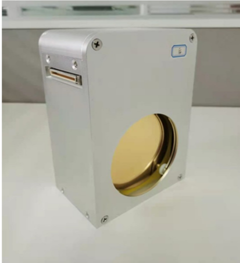
Figure 4: A MLFC prototype consists of 128 layers sheet.
