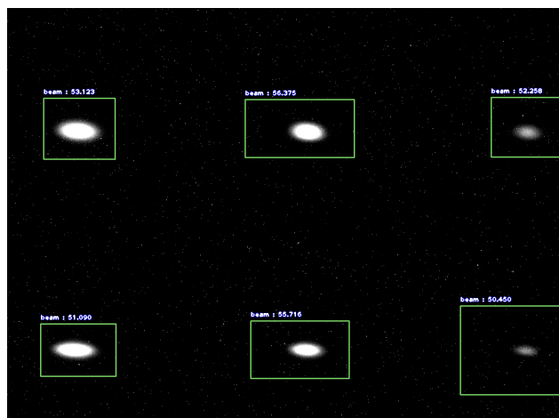
Figure 8: A single pinhole CCD frame with 6 beam spots detected by a trained YOLO model.
