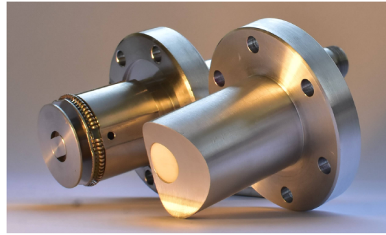
Figure 3: On the left, the longitudinal section of a ChDR button. The ceramic and metal part are indicated. On the right, a picture of a ChDR button (front), compared to a traditional capacitive BPM button (back). The white ring is the ceramic insert in the metal button.
