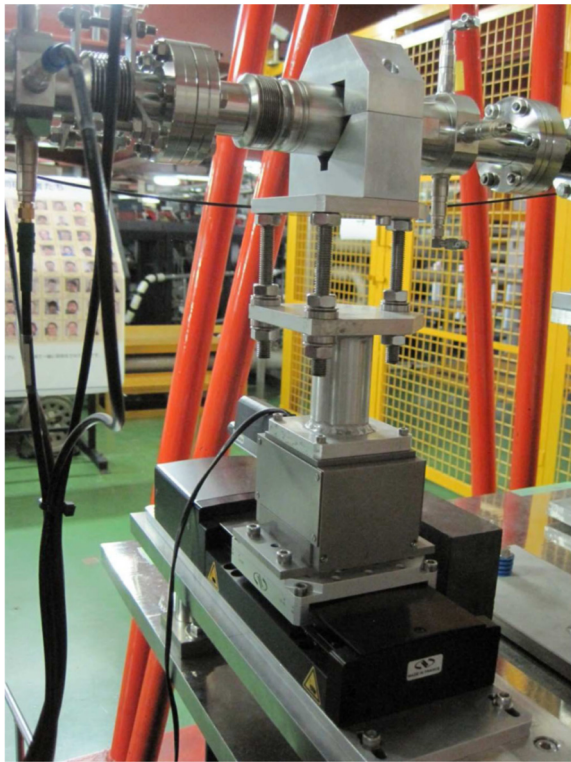
Figure 3: Photograph of FONT5 stripline BPM P3 and its mover in the ATF2 beam line.
