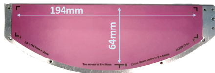
Figure 3: SBDS Al 2 O 3 :CrO 2 screen mounted on its support, ready for installation.
