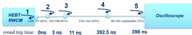
Figure 6: Cabling between the HEBT RWCM and the oscilloscope (inspired by D. Frolov's drawing).
