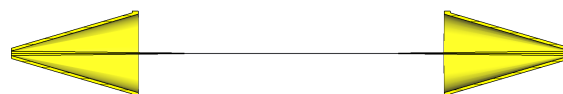
Figure 1: Schematic of a Goubau-line consisting of two conical horn antennas and a dielectrically coated wire similar to the design at Argonne APS [9].
