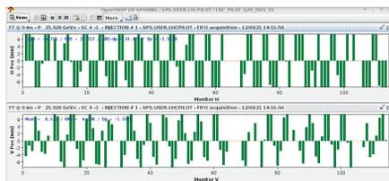
Figure 2: A screen capture of the SPS BPM operational software depicting the first successful injection in the accelerator as captured by ALPS in FIFO mode. The trajectory measured made it possible to promptly correct the optics settings.
