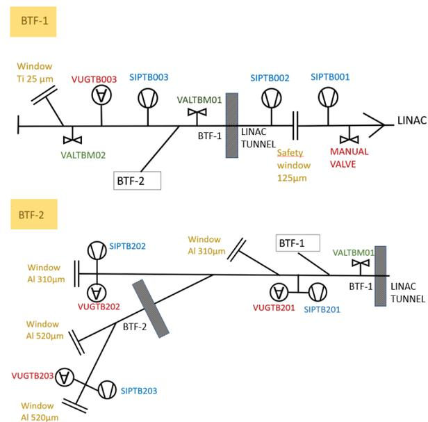
Figure 3: The BTF Vacuum system layout.
