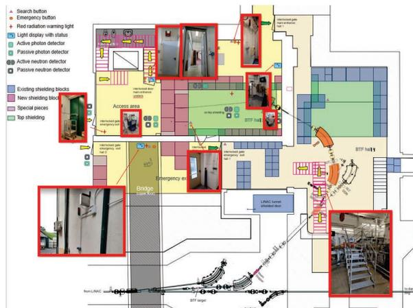
Figure 5: The layout of the BTF2 safety system.
