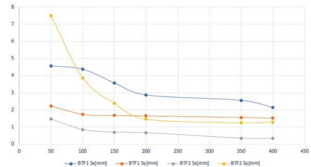
Figure 11: The plot of the measured BTF2 and BTF1 beam size vs Energy.
