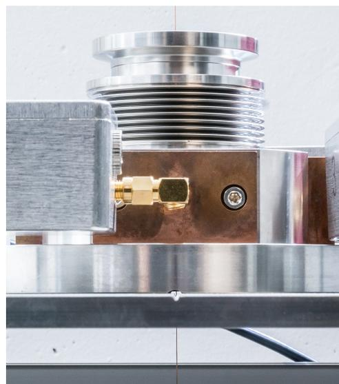
Figure 3: V-groove for wire positioning.
