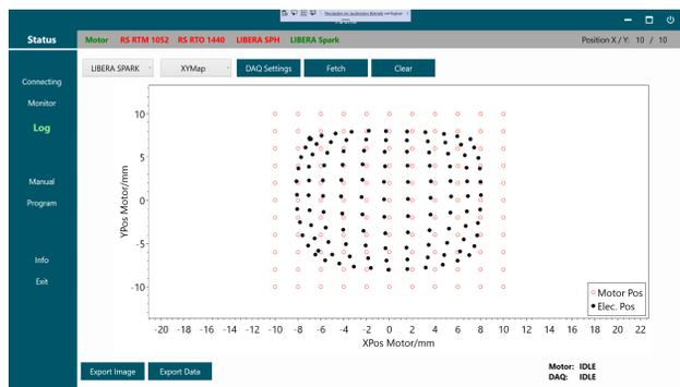
Figure 4: Screenshot of a TBens data acquisition window showing a 2D response map.
