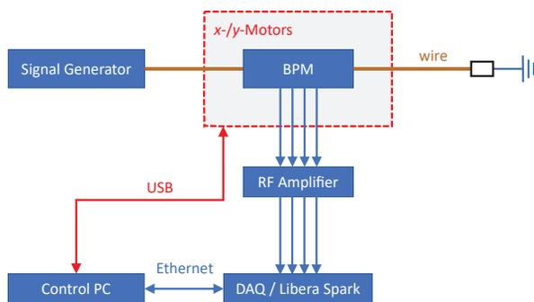
Figure 2: Schematic layout of the BPM test bench cabling.
