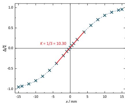
Figure 5: Exemplary BPM sensitivity measurement with a linear fit for the centre region (red).
