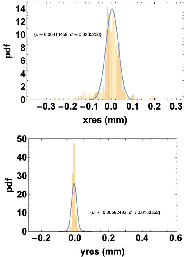
Figure 3: Resolution of the position measurement in DBP02 in horizontal (top) and vertical.
