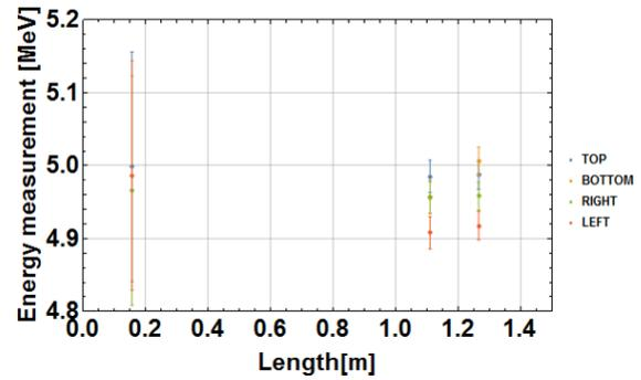
Figure 6: Energy measured at the DPLA for a 24 mA deuteron beam with the first digitizers.
