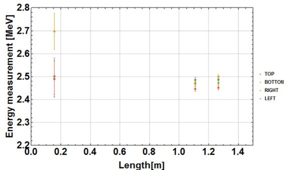
Figure 5: Energy measured at the DPLA for a 52 mA proton beam.
