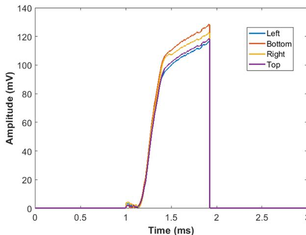
Figure 2: Example of evolution of the amplitude measurement of the four electrodes of a BPM during a single beam pulse.
