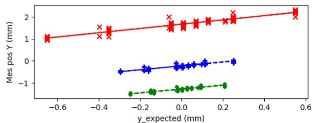
Figure 4: Horizontal steering tests of the DPLA BPM's: D1 (green), D2 (blue) and D3 (red).
