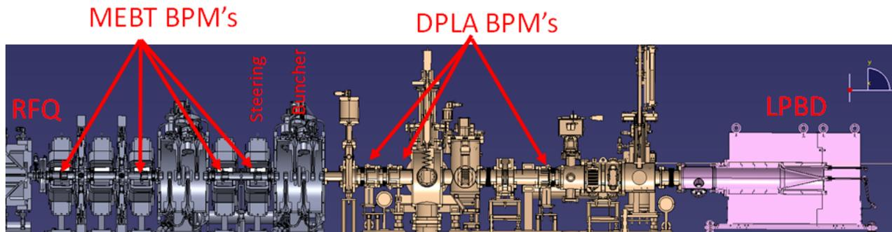
Figure 1: Layout of the LIPAc Phase B1/2 for RFQ and MEBT proton and deuteron pulsed commissioning.
