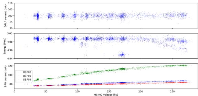
Figure 7: Evolution of the beam current, beam energy and BPM current during a voltage scan of the second buncher cavity for a 100 mA deuteron beam using the upgraded electronics.
