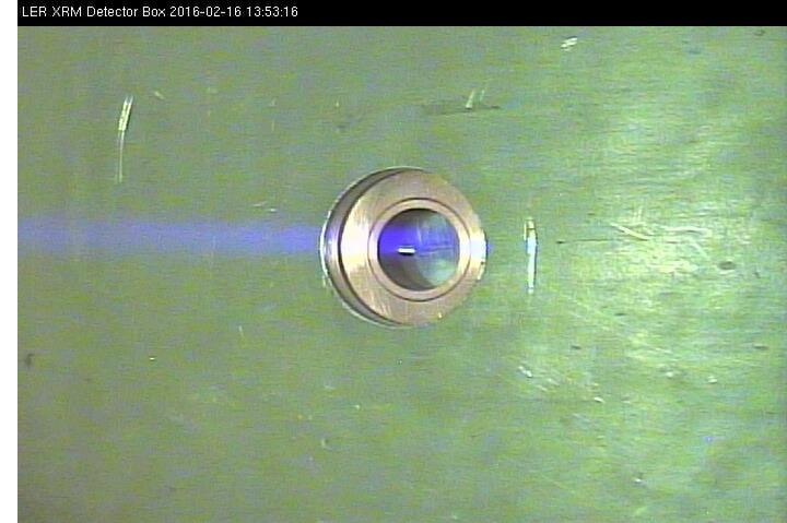
Visible x-ray path in air (LER, 100 mA):
