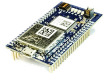
open source RFFE- \mu C board designed at LNLS
