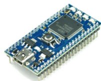
commercial mbed microcontroller board
