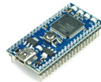
commercial mbed microcontroller board
