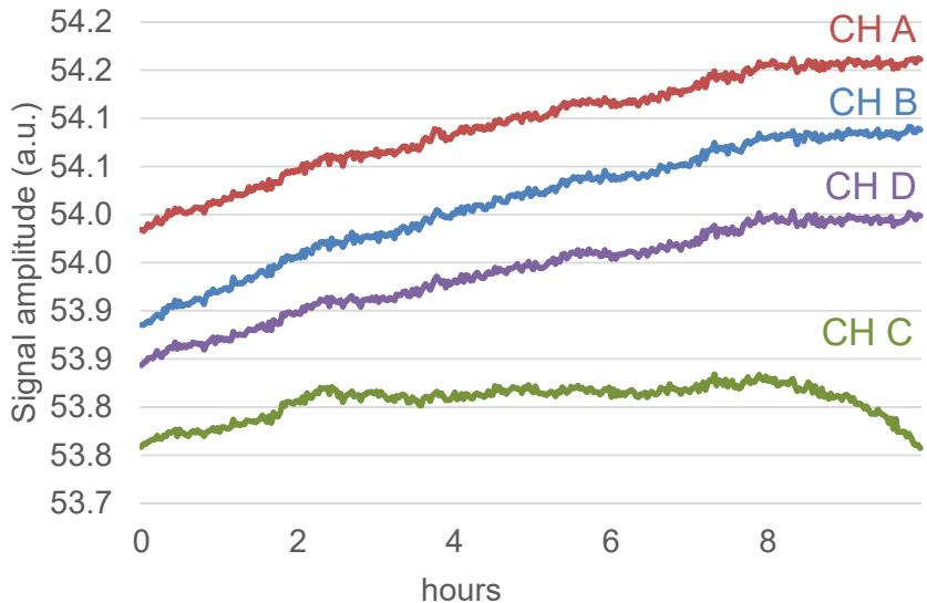
The common reference voltage for the ADCs had a broken contact: so ADC C was using the internal reference voltage rather than the common external one, causing the unexpected drift.
