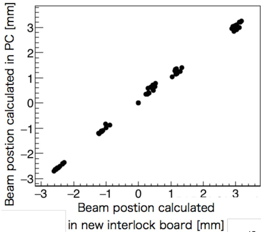
**Confirmed that the beam position calculation in the new board is consistent with one calculated in PC**
