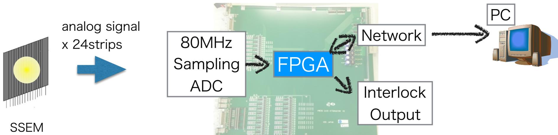
(1) calculate an integrated charge of each strip
