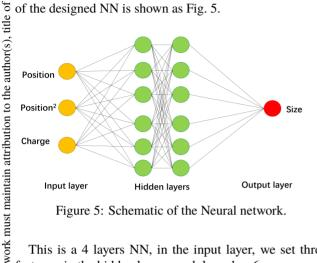
This is a 4 layers NN, in the input layer, we set three features, in the hidden layers, each layer has 6 neurons, we choose 'tansig' as the transfer function; the predicted beam size value can be obtained from the output layer; Levenberg-Marquardt is used as the training algorithm.
