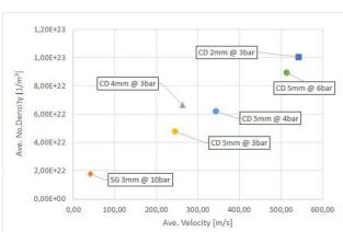
Figure 2: Comparison between nozzle geometries for different nozzle throat to skimmer distances (mm) and inlet pressures (bar).
