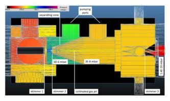
Figure 3: TPMC model showing main components and corresponding pressures.
