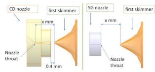
Figure 1: Nozzle and first skimmer as used in the simulations, with x the variable distance between the nozzle throat and the opening of the first skimmer.
