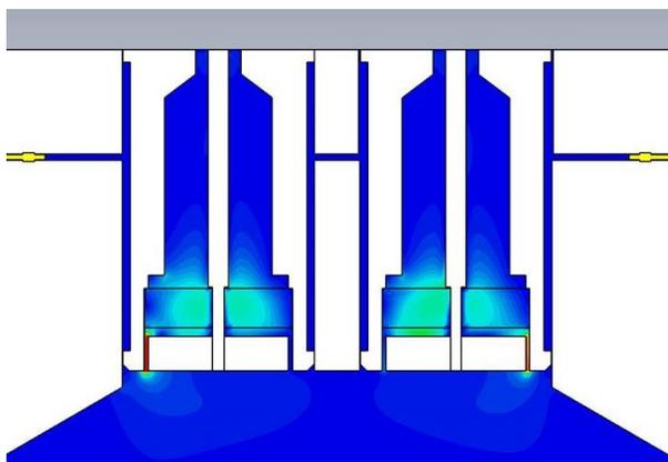
Figure 3: Computed electric field distributions of the trapped mode in aluminum oxide insulator of original button BPM at BESSY II.
