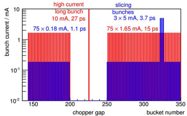
Figure 1: Section of a possible filling pattern with short bunches (blue) and long bunches (red). Trains of short bunches are added to supply THz power as well as high repetition rate short x-ray pulses.
