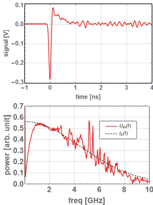
Figure 2: Measured single-bunch signal with the beam current of 1 mA (top) and the frequency spectrum of the signal (bottom) from the BESSY II button BPM. The curve named  $U_{im}$  is the Fourier transform of the measured signal and  $I_b$  is the spectrum of a Gaussian beam.
