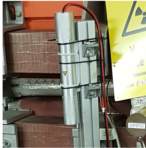
Figure 3: BLM prototype based on a scintillator and PMT setup during tests in the COSY synchrotron.
