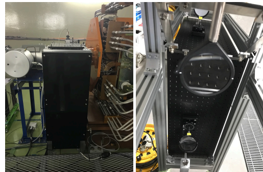
Figure 7: Optic system with frame installed in J-PARC neutrino beam line with front view (left) and inside with two lenses and 45° downward-mounted mirror (right).
