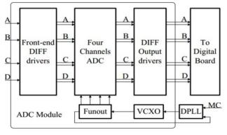
Figure 4: ADC module of DBPM processor.
