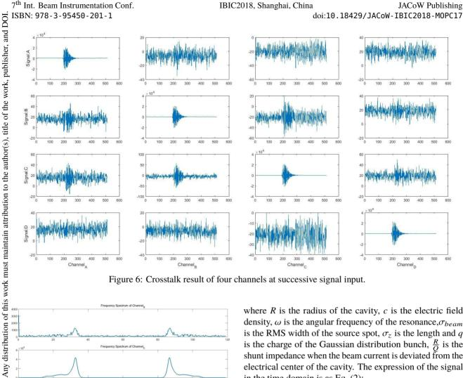
Figure 6: Crosstalk result of four channels at successive signal input.
