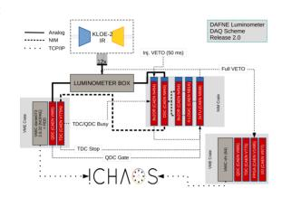
Figure 2: Schematic view of the DAQ acquisition. The signals coming from a corresponding sectors on the two sides are compared with a fixed threshold and used to measure arrival time and integrated charge when the trigger logic condition is fulfilled.
