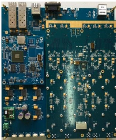
Figure 4: Photography of the current BPM signal processor on SXFEL.
