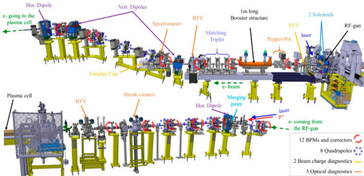
Figure 1: AWAKE beam lines and BPM locations.
