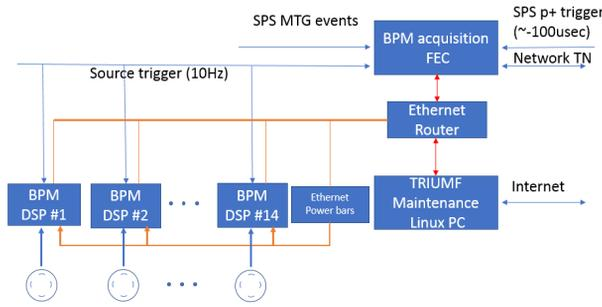
Figure 2: AWAKE stripline BPMs: electronics, triggers, DAQ, and Maintenance computers.
