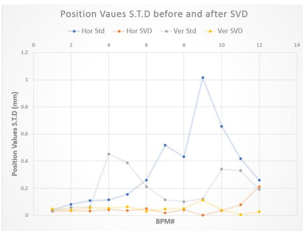
Figure 8: Beam position STD before and after SVD.
