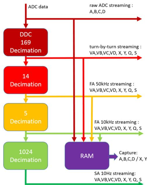
Figure 1: DBPM signal processing diagram.
