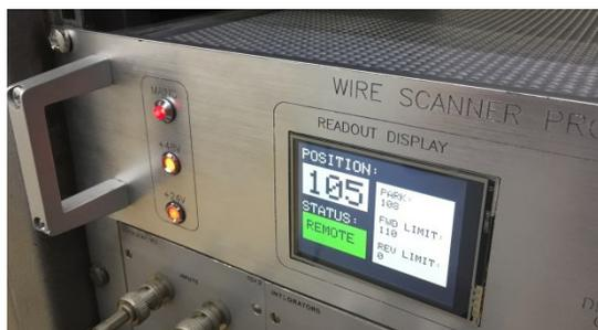
Figure 4: Motor control unit readout display.
