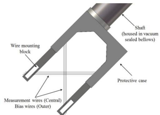
Figure 1: Orientation of a wire scanner head, with a signal wire and pair of bias wires mounted in each plane.
