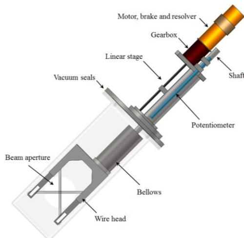
Figure 2: Simplified layout of the profile monitor.
