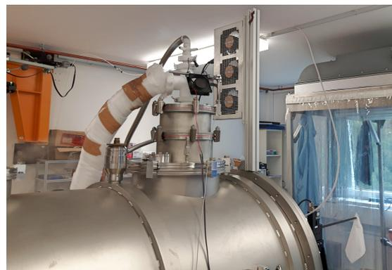
Figure 8: The cryomodule of Gun III during cooling with liquid helium.
