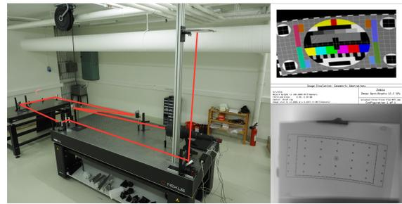
Figure 9: Prototype of the optical system at the University of Oslo. The image target is shown on the bottom right, and the Zemax simulation on the top right. The agreement shows that the performance in design and in reality are matched.
