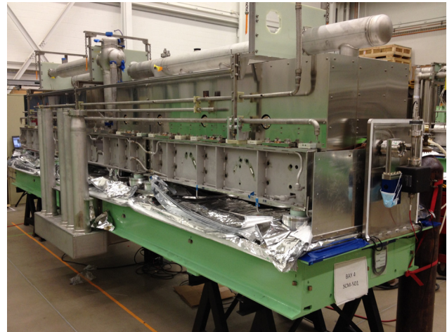
Figure 7: Pre-production \beta_0=0.53 cryomodule under assembly, with 8 SRF cavities operating at 2 K and a solenoid operating at 4.5 K temperature, respectively.
