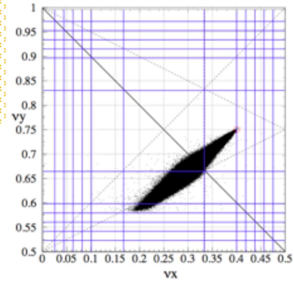
**The observed peak indicate existing the resonance oscillation induced by the quadrupole kicker.**
