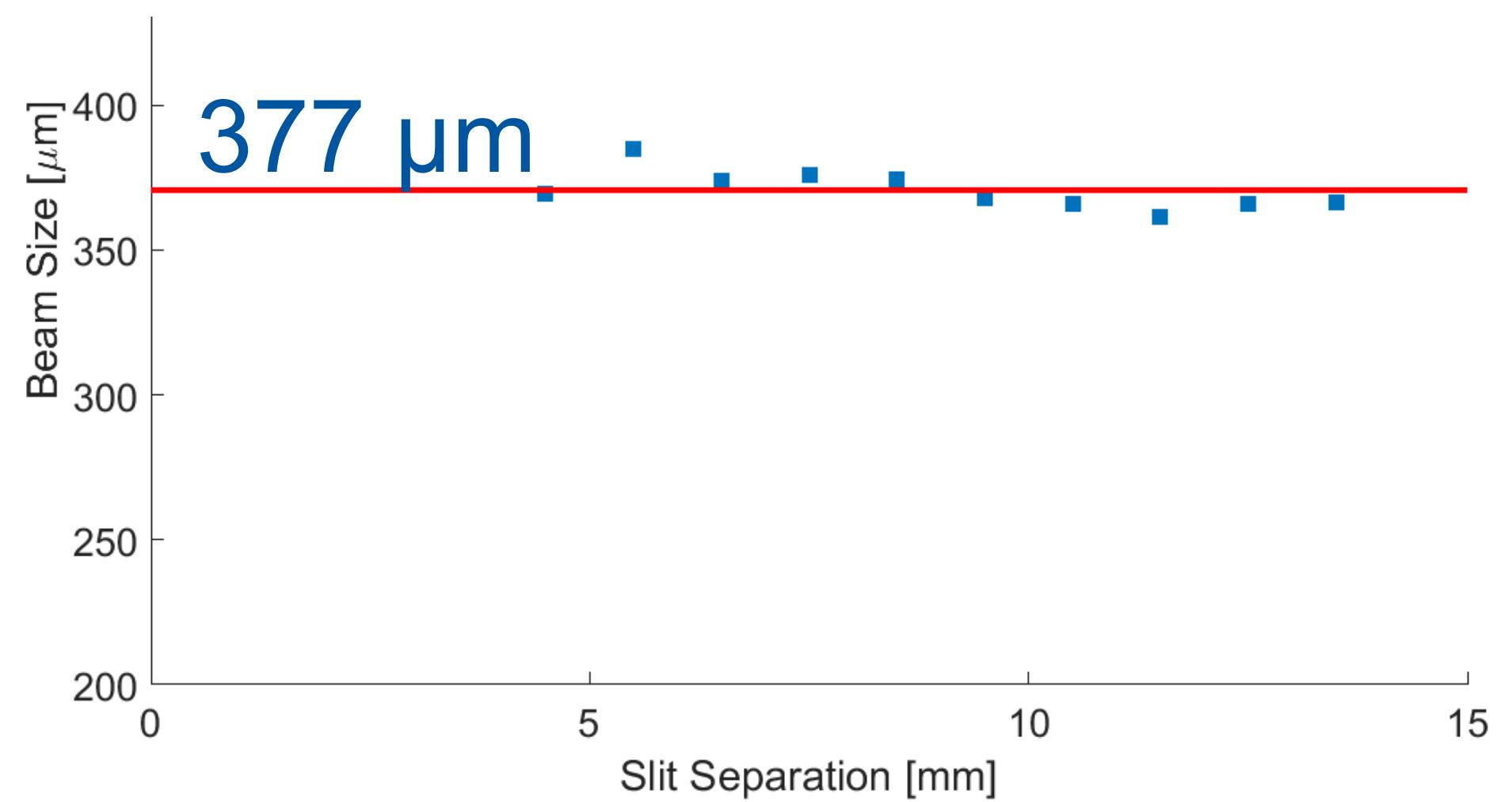
Beam Size:  $\sim 375 \mu\text{m}$
