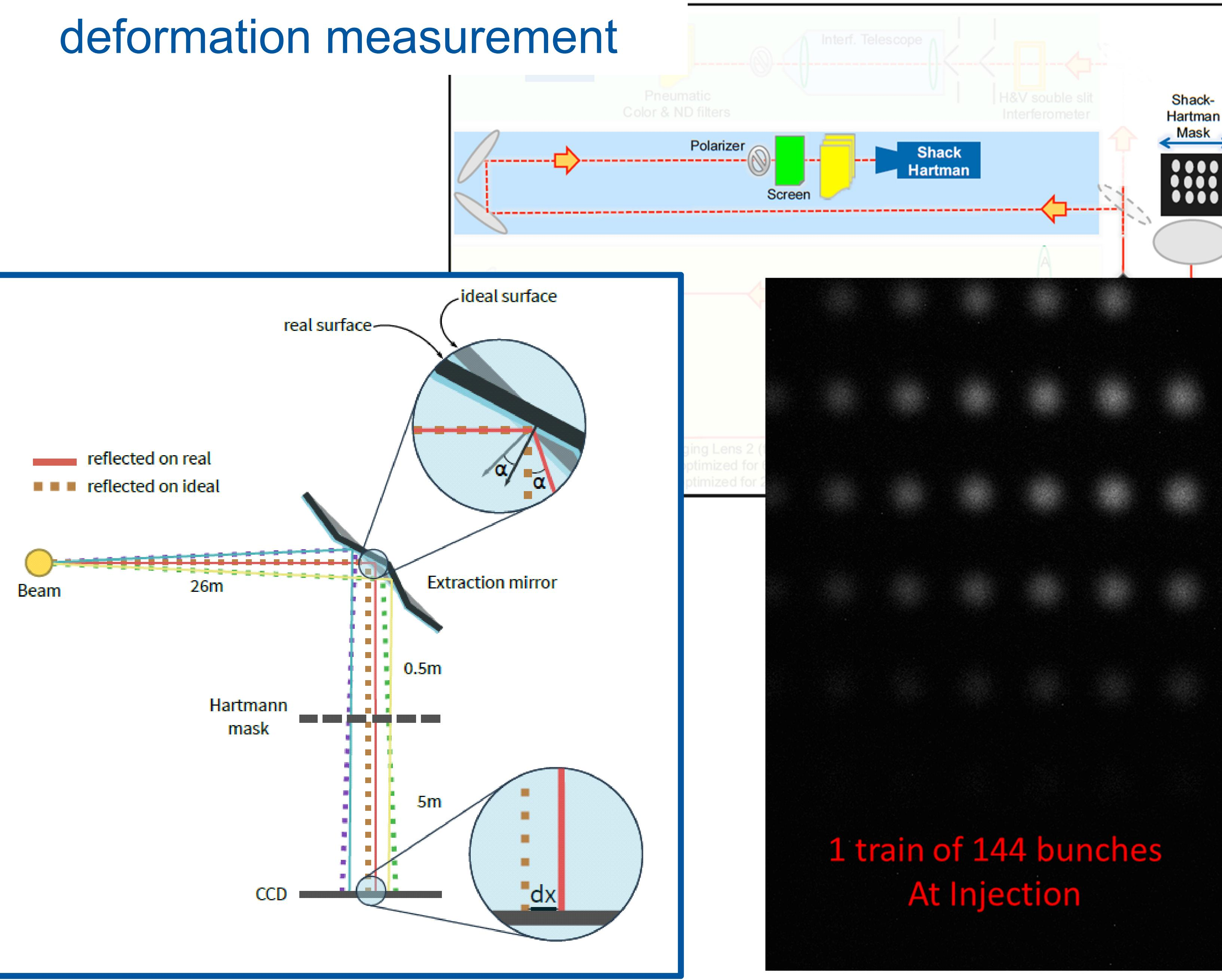
No deterioration of the extraction mirror surface flatness is caused by the full intensity circulating beam.
