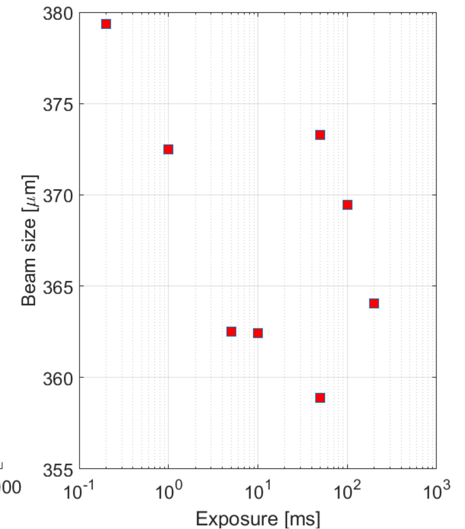
The measured beam size, 366 (MEAN)  $\pm$  5,6  $\mu\text{m}$  (RMS),
