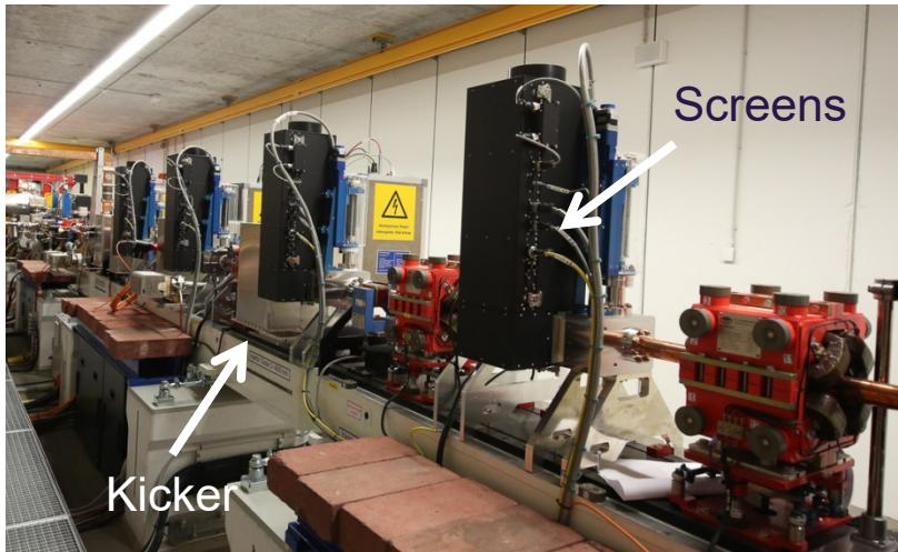
These measurements are fast (2.5 Hz) and allow also to measure the emittance and their evolution over the bunch train.
