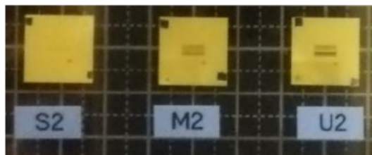
Masks: \sim 20 \mu\text{m} Au on 600 \mu\text{m} CVD diamond substrate
