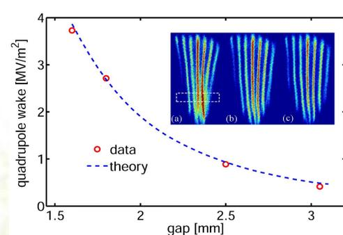
Measured (red circles) and simulated (blue dashed line) quadrupole wake fields of the central slice at various gaps. The streaked beamlets at various CS gaps are shown in the insets [(a) for  $g = 3:6$  mm, (b) for  $g = 5:0$  mm and (c) for  $g = 6:1$  mm]. The dashed square indicates the region of the central slice used for analysis.
