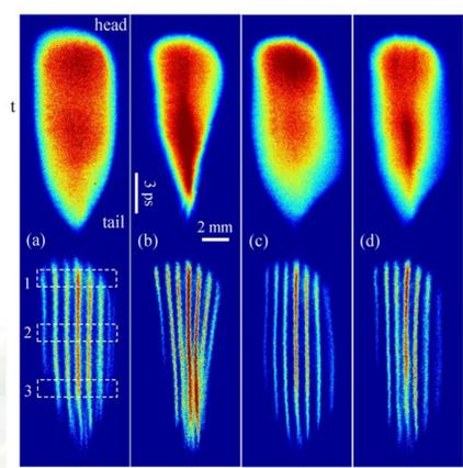
Time-resolved measurements of beam (top) and beamlets (bottom) distribution on screen P1. Four situations are shown: (a) with two CS widely open; (b) with downstream CS gap set at 3 mm; (c) with upstream CS gap set at 3 mm; (d) with both CS both gaps set at 3 mm. The dashed squares in (a) indicates the three representative slices used for analysis of emittance and phase space
