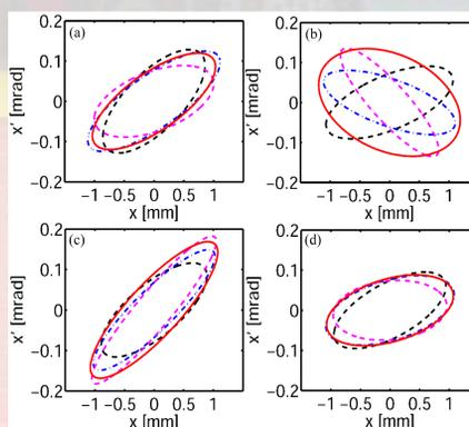
Slice and projected phase space ellipses in four situations: (a) with two CS widely open; (b) with D CS gap set at 3 mm; (c) with U CS gap set at 3 mm; (d) with both CS gaps set at 3 mm. The phase spaces for the head slice, central slice and tail slice are shown with dashed black line, dotted dashed blue line and dashed magenta line, respectively. The projected phase space is shown with solid red line.
