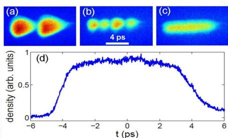
Time-resolved measurements of beam distribution at screen P1 with (a) 1 crystal, (b) 2 crystals, and (c) 3 crystals; the corresponding beam current distribution with 3 crystals inserted is shown in (d).
