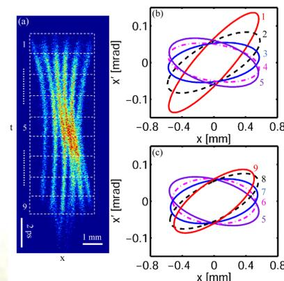
(a) Streaked beam distribution with the gap of the downstream CS reduced to 1.4 mm; (b) Phase space ellipses for the front five slices (from bunch head to bunch center); (c) Phase space ellipses for the latter five slices (from bunch center to bunch tail).
