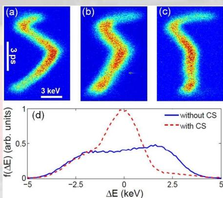
Time-resolved measurements of beam longitudinal phase space distributions (bunch head to the up) at screen P2 (a) with the two structures open, (b) with one of the CS gap reduced to 3 mm, and (c) with the gaps of the two CS both set at 3 mm; (d) the corresponding projected beam energy distribution.
