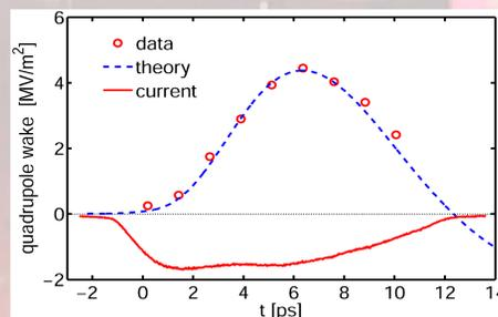
Measured (red circles) and simulated (blue dashed line) time-dependent quadrupole wake fields with the gap of downstream CS set at 3 mm. The beam longitudinal distribution is also shown in red solid line.
