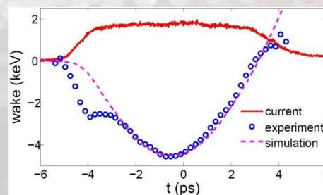
Measured and simulated longitudinal wake potential of the CS. The bunch distribution, with the head to the left, is also shown with the red line.
