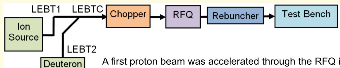
A first proton beam was accelerated through the RFQ in December 2015. In the first semester of 2016, the commissioning was done with proton and helium beams in pulse and CW mode.
