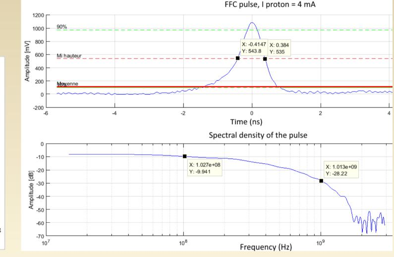
FWHM: 800 ps, σt calculated from the pulse = 328 ps, σt simulated with tracewin = 220 ps
