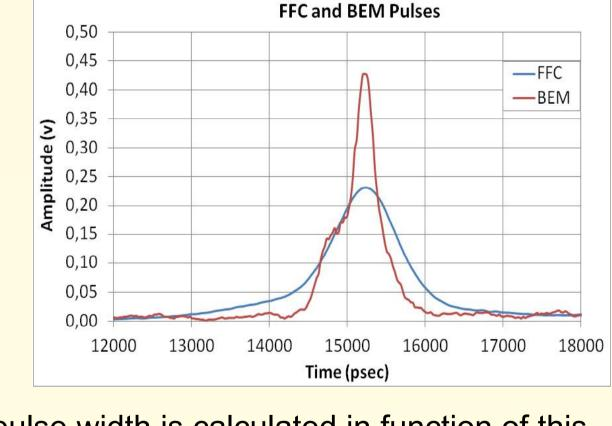
At 75kV, the rebuncher phase is shifted on 360°, the pulse width is calculated in function of this phase.  $\sigma t = f (\varphi rebuncher)$
