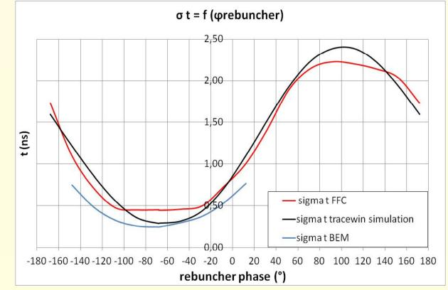
The FFC curve shows a limitation in time. The minimum value of  $\sigma t$  is equal to 440 ps.
