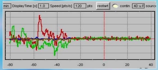
**Left:** Stabilisation system off and subsequently turned on. Red and green lines are the angle and position value respectively (arbitrary units on y-axis)
