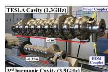
Each cavity has 9 cells. RF power is input through the power coupler, while the HOM power generated by the beam is extracted through 2 special couplers mounted in the beam pipes at either end. 8 cavities are mounted in one cryo-module
