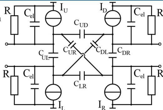
Equivalent Circuit of a capacitive pickup with four electrodes. Each electrode is capacitively coupled to one another and to GND.
