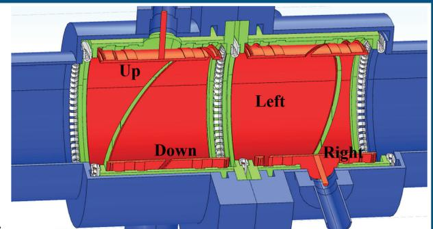
Simplified Comsol model of the diagonally cut BPM for capacitance determination. Blue; beam pipe, green; grounded housing cylinder, red; electrodes. BPM plane length (e.g. Up + Down) 77mm, radius 44.5 mm.
