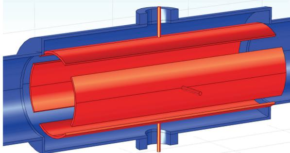
Simplified model of the quad strip type BPM. Blue; beam pipe, red; electrodes. Length 270 mm, radius 44.5 mm, angular cover  $70^\circ$  each.
