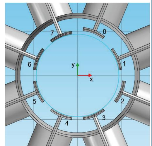
Conceptual model of an eight strip beam size monitor. Electrode 0 and 2 are shifted straight along the x and y axis. Two electrodes are shifted to obtain multiple electrical centers and thereby different drifts of faulty beam positions.
