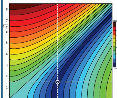
Colour coded plot of standard deviations of beam positions of various electrode configurations. The isoline plot can be obtained and quantified analytically or by test bench measurements.
