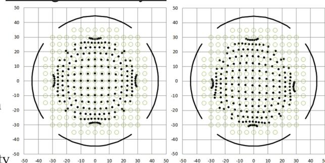
Projection plots of an ideal and a misaligned BPM. These plots show where the beam would be projected, if the simple linear response is assumed.
