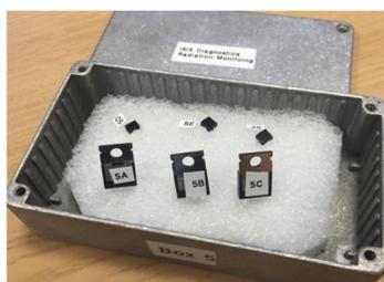
The measured diode and FET voltage increased more in areas that have more beam losses and radioactivity.
