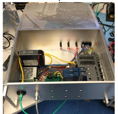
The data acquisition is done by a National Instruments cRIO that is cabled to the sensor board from a shielded area.
