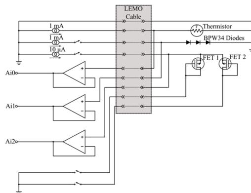
RadFETs, pin diodes and a thermistor are used in the measurement system to log dose and temperature.
